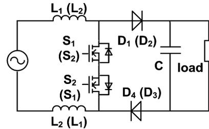
Fig. 5. Simplified topology for symmetric bridgeless PFC in half-line cycles.
