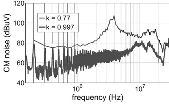
Fig. 11. Effects of coupling coefficient on CM noise.
