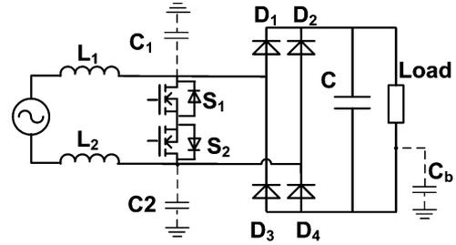
Fig. 4. Symmetric topology of bridgeless PFC converter (re-organized).
