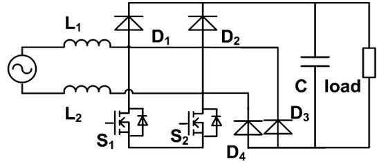
Fig. 3. Symmetric topology of bridgeless PFC converter.
