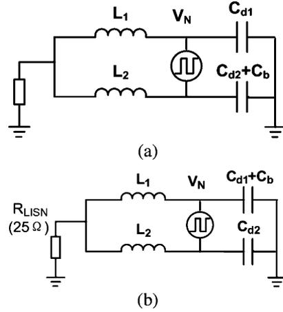
Fig. 13. CM noise models of bridgeless boost PFC for two half-line cycles: (a) positive half-line cycle and (b) negative half-line cycle.
