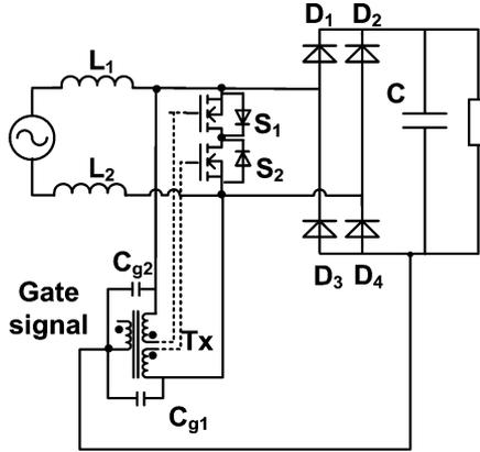
Fig. 8. Improved symmetric bridgeless PFC with gate drive transformer.
