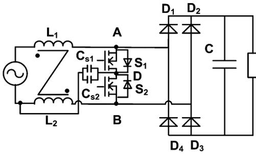
Fig. 9. Improved symmetric bridgeless PFC with heat-sink connected to power line.
