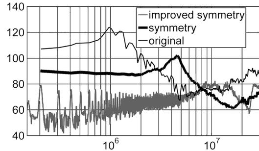
Fig. 16. CM noise comparison between original, symmetric and improved symmetric bridgeless PFC.
