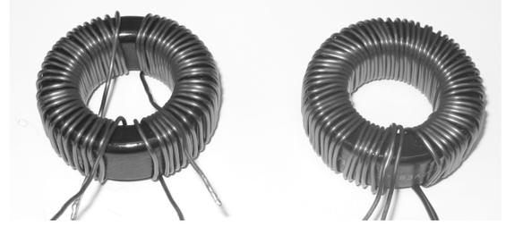
Fig. 10. Coupled boost inductors with different winding techniques (1:1 turn ratio).
