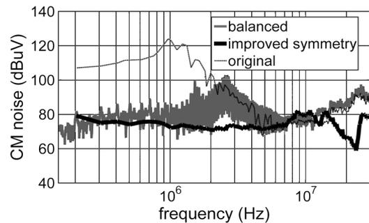
Fig. 17. CM noise comparison between original, improved symmetric and balanced bridgeless PFC.
