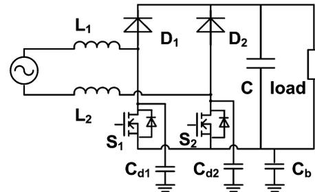
Fig. 1. Topology of bridgeless PFC with parasitic capacitances to ground.
