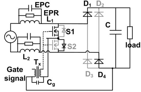
Fig. 7. Positive half-line cycle with parasitic effects.
