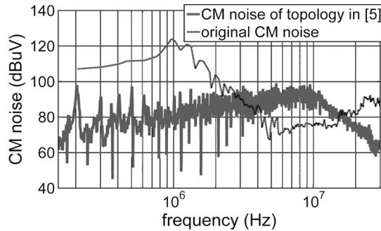
Fig. 15. CM noise comparison between the original bridgeless PFC and the topology proposed in [5].
