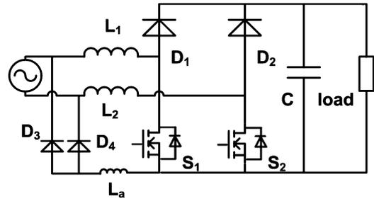
Fig. 14. Bridgeless PFC using balance technique.
