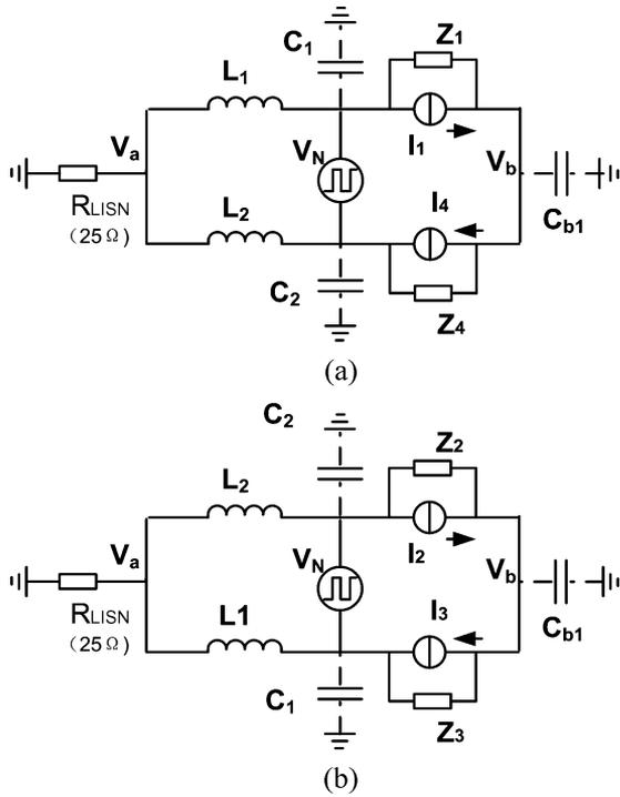
Fig. 6. CM noise model for symmetric bridgeless PFC in half-line cycles: (a) positive half-line cycle and (b) negative half-line cycle.
